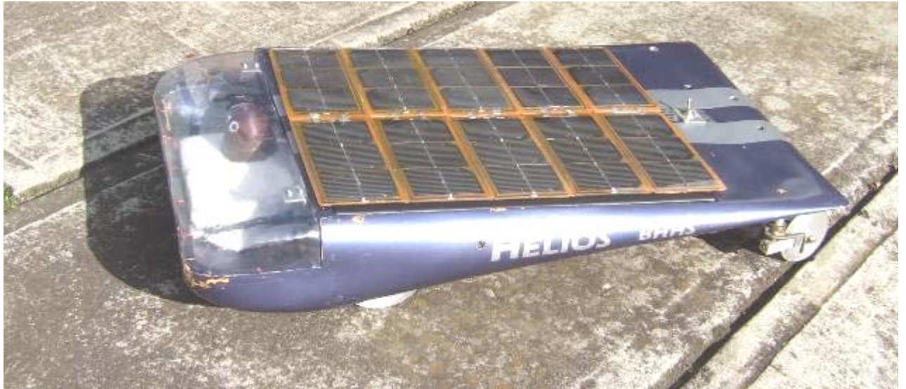
HELIOS : SIMULATOR AIR DRAG COEFFICIENT 0.004 (Note: This car designed to meet the 200 sq.cm. transverse panel requirement.)
