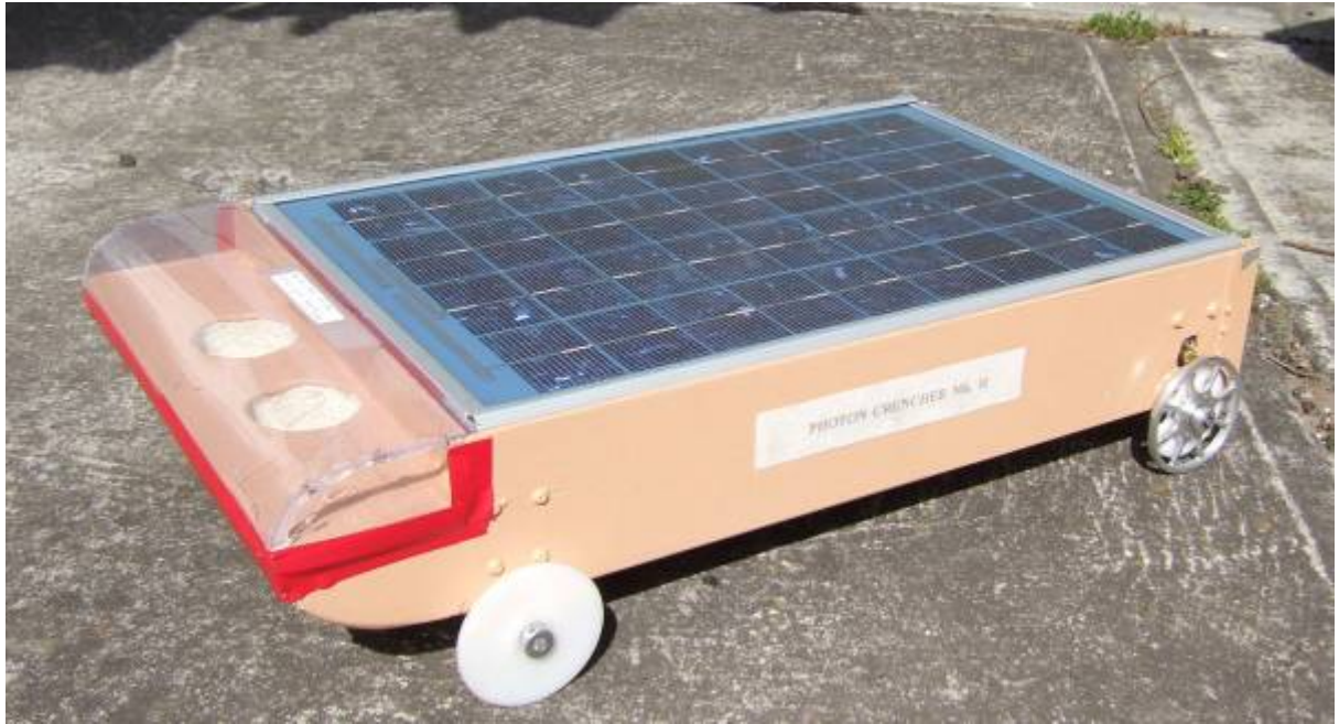
PHOTON CRUNCHER MK II : SIMULATOR AIR DRAG COEFFICIENT 0.012 (Note:This car designed to meet the 200 sq.cm. transverse panel requirement.)
