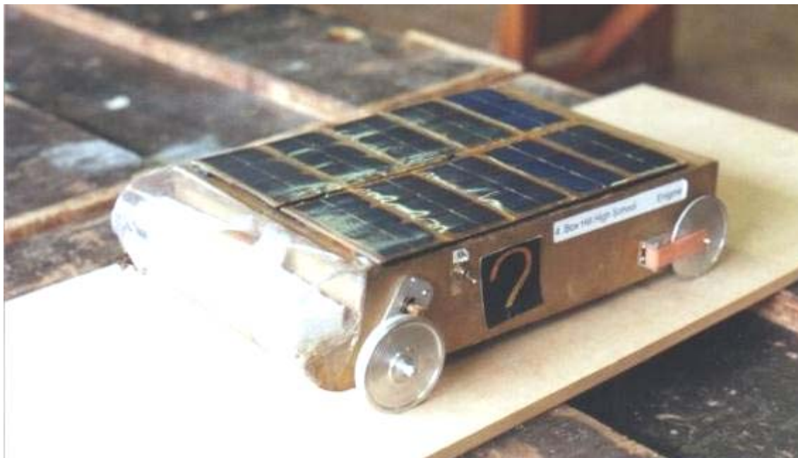
ENIGMA : SIMULATOR AIR DRAG COEFFICIENT 0.012 (Note:This car designed to meet the 200 sq.cm. transverse panel requirement.)
