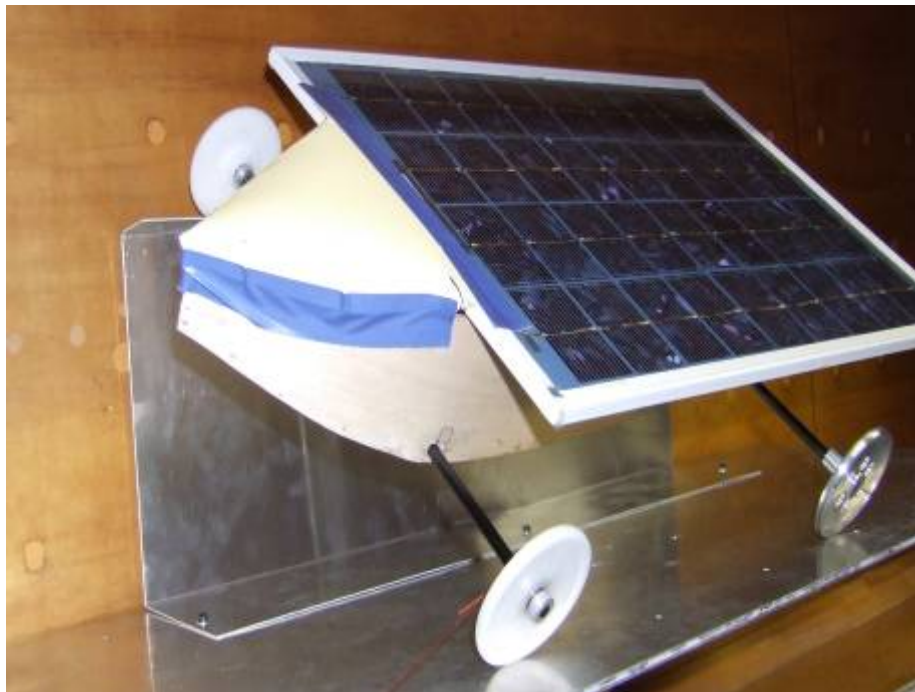
SYNDAL SOUTH 2006 CAR : SIMULATOR AIR DRAG COEFFICIENT 0.0045
