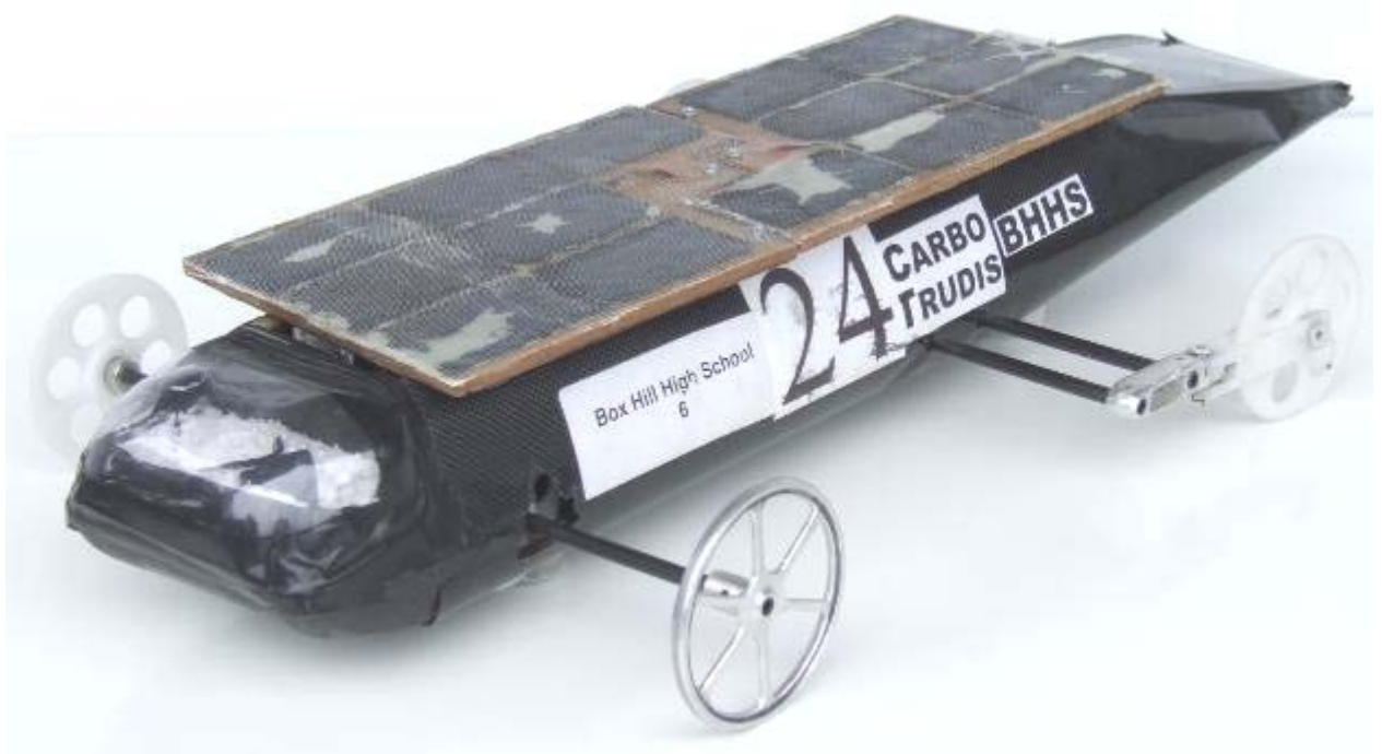
CARBO TRUDIS: SIMULATOR AIR DRAG COEFFICIENT 0.0039
